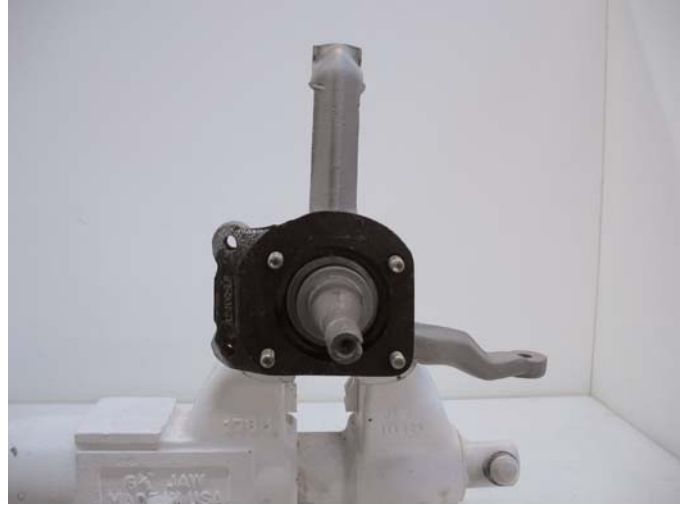
Insert 3/8" mounting bolts from the rear and install the bracket over the front of the spindle.
