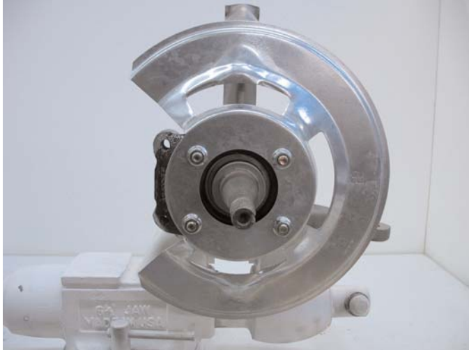
Install the splash shield over the spindle onto the mounting bolts. Secure with 3/8" nuts. Torque to 35-45 ft-lbs.
